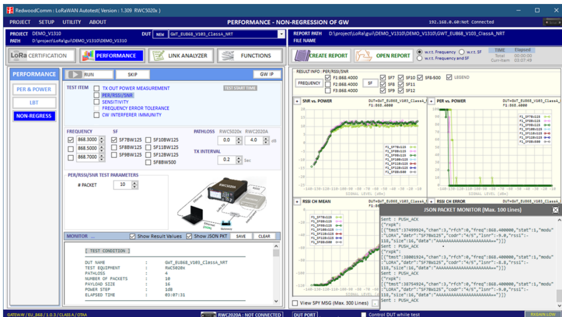
Fig 3.22 Non-regression test control and parameters window
