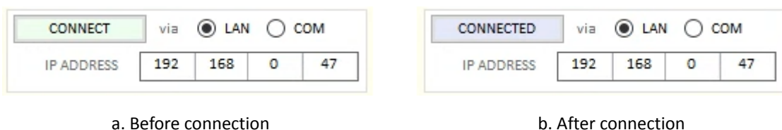
Fig 2.12 Make a connection between PC and RWC5020x/5021x via LAN
