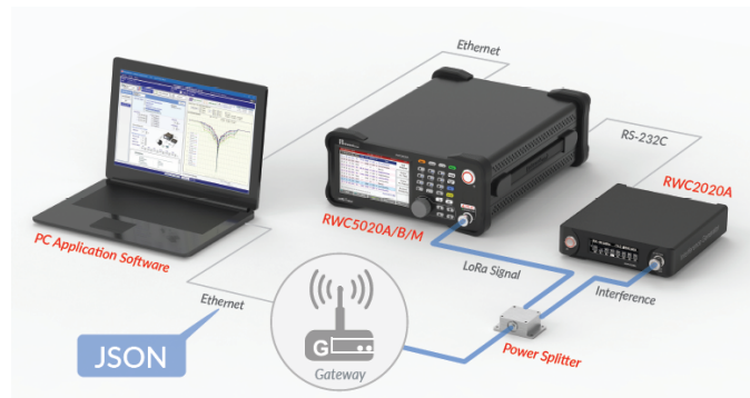
Fig 3.24 The Concept of non-regression test of gateways
